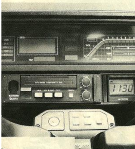
Motorcycle instrumentation reaches new heights—analogue and digital LCD readouts monitor vital signs on the Voyager. Most are standard fare for big touring bikes, but the compass (left of radio) is a new touch. It uses a sensor set on the front fender, declination adjustable. Controls right of the ignition include cruise lean-out for the DFI.
