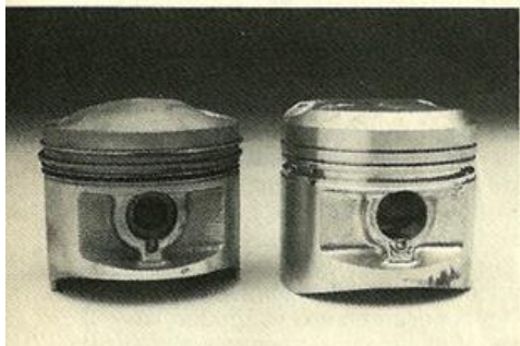
The new Voyager uses flat-crown pistons (right) that have a clear squish band. Old, low-dome piston is on left. Flat-top piston aids flame propagation.
