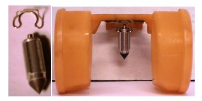
The manual for the Voyager shows the setting of the float as 17mm, yet I find these settings result in too high a fuel level. I set my floats 1mm lower (18mm) to compensate yet will show 17mm.
