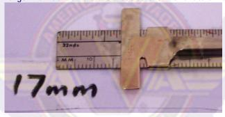
Place the carbs on their side so the float is not pressing on the float valve, find the point where the float just touches the valve without depressing the spring. This position should be 17mm from the bottom of the float to the gasket surface on the carb. Do not make this setting with the float resting on the valve!
