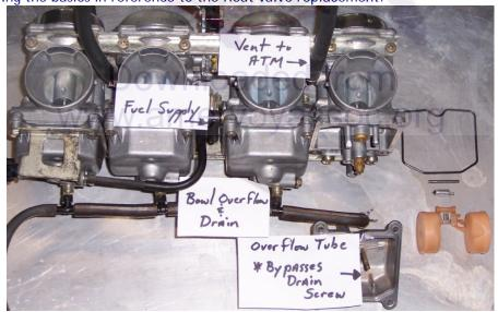
First step is to remove all four bowls, slide out the float pin, and lift out the float and valve. Please keep in mind I suggest taking the entire carb apart for a full clean, then reassemble. For the sake of this write, I will only talk of the bowl area.
