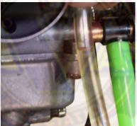
Open the drain screw to allow fuel to fill the tube, then slowly lower the tube to get an accurate reading. The fuel level spec is 0.5mm below the top of the bowl, +/- 1mm. Check all four and adjust if necessary.
