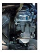
Now, another major issue! The manifolds from the Airbox to the carbs. There are springs that are used to secure the manifolds to the carb. These will be, just rolled back, to remove the tension on the rubber collars. (This is easy) However, reinstalling will require you to be able to roll these springs up, onto the manifolds. (I used both, my fingers, and some dental tools to finess these compression springs
