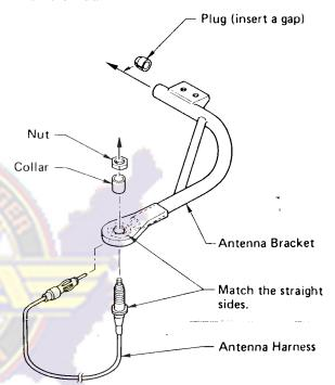
Attaching the Antenna Bracket to the Chassis
