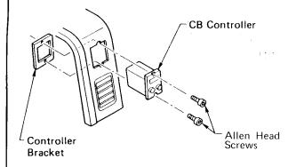
Attachment of the Bracket to the CB Main Unit
